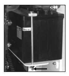
Figure 28: Battery Support Brace
